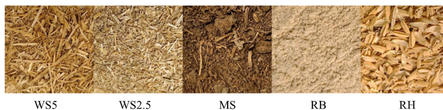
Fig. 2 – Appearance of some reinforcement components used in the blends. From left to right, wheat straw sieved at 5 mm (WS5), wheat straw sieved at 2.5 mm (WS2.5), used mushroom substrate (MS), rice bran (RB) and rice husks (RH).
