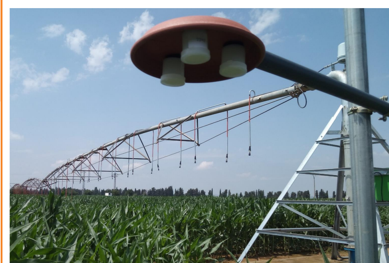
ALPHA samplers placed in the pivot monitored in Cinco Villas (Spain)
