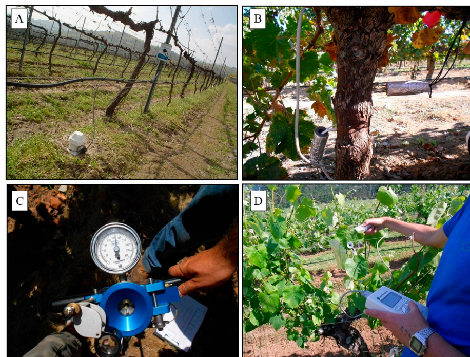
Figure 3. Devices for the assessment of grapevine water status: (A) Soil capacitance probe for continuous monitoring of soil water content; (B) Sap flow probe in the trunk of a grapevine; (C) Pressure chamber; (D) Hand-held porometer for determining stomatal conductance. Photos were taken by J.M. Mirás-Avalos.
