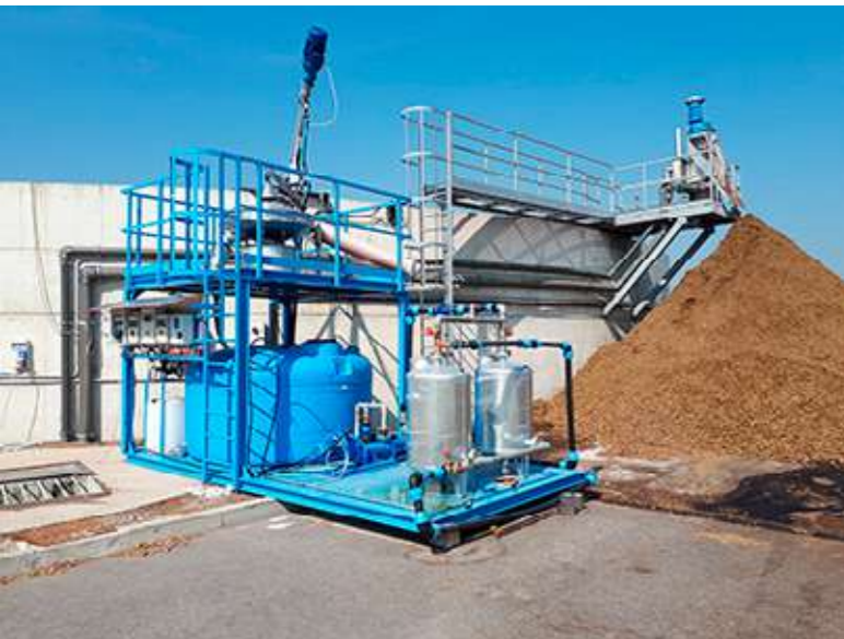
Image 6.2. Filtration system installed to supply the digestate to the drip irrigation in the Drip 1 farm in Lombardy (Italy).
