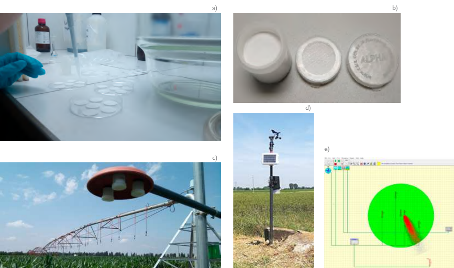
Image 4.4. APS filter preparation in the laboratory, b) ALPHA ® sampler, c) ALPHA ® samplers placed in the field, d) meteorological station and e) WindTrax simulation software.
