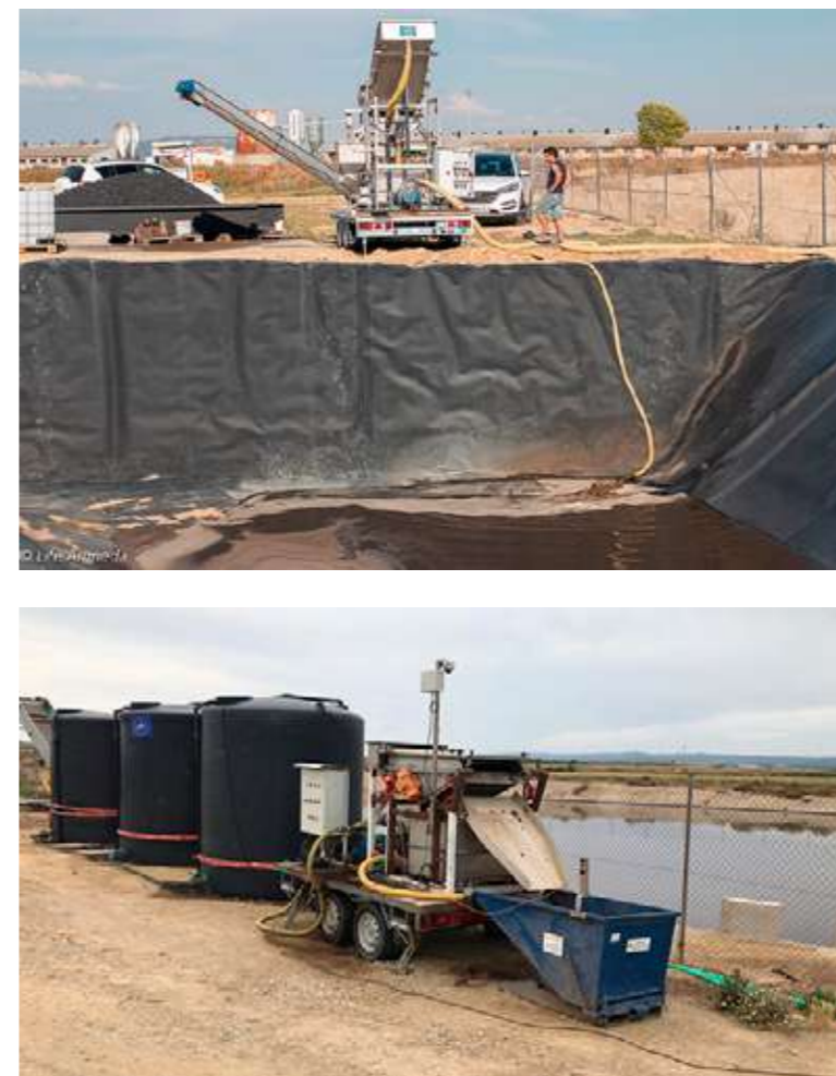
Image 5.1. Solid/liquid separators, pivot prototype (up) and drip prototype (down) in Farm 1 (ES-S1-F1) that provided liquid fraction for demonstration field at Torremira in Cinco Villas (ES-S1-D).
