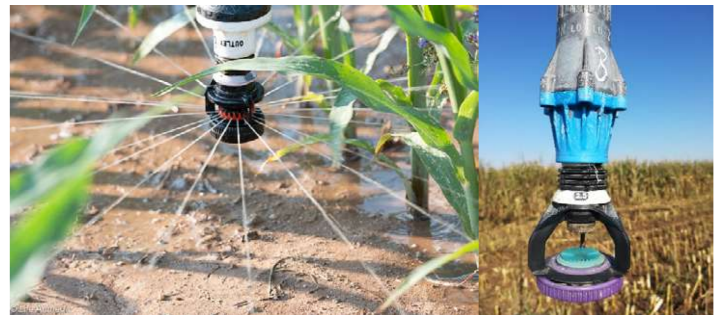
Image 3.11. Irrigation nozzles installed in LIFE ARIMEDA pivots demonstration fields in Aragon (left) and Lombardy (right).
