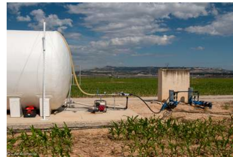
Image 4.9. Instruments for volume injection control in the drip irrigation plot fertigated in Cinco Villas.
