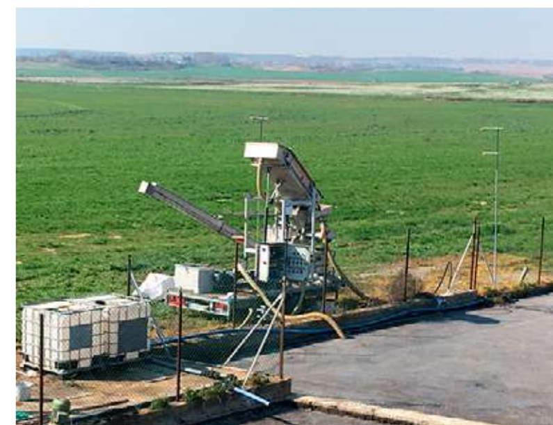
Image 5.2. Solid/liquid separator for pivot and liquid fraction storage pond at Farm 3 (ES-S2-F3) that provided liquid fraction to demonstration fields at La Melusa in La Litera (ES-S2-P, ES-S2-D).
