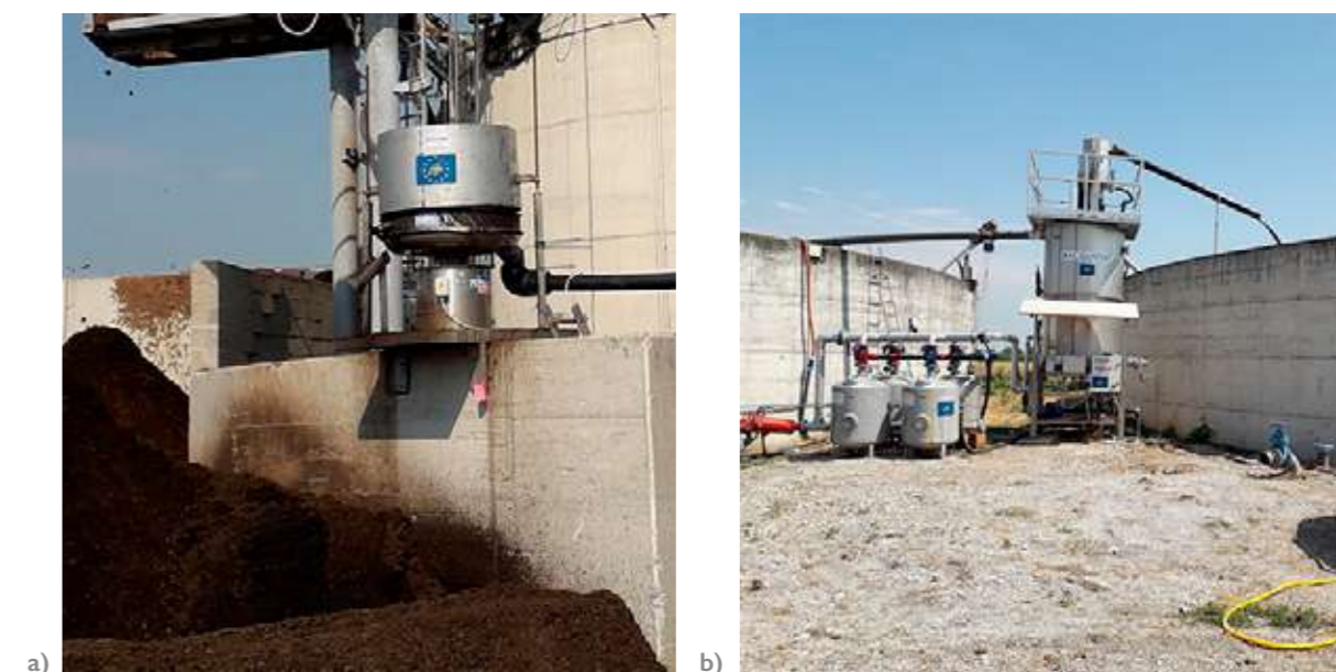
Image 6.1. Vibrating screen (a) and microfilter (b) used for filtration of digestate in Lombardy (Italy).
