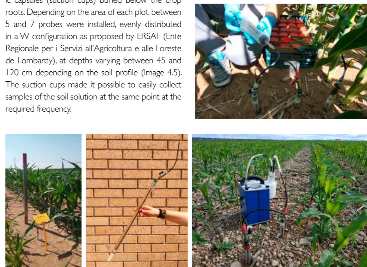
Image 4.5. Ceramic suction cups installed in LIFE ARIMEDA plots..
