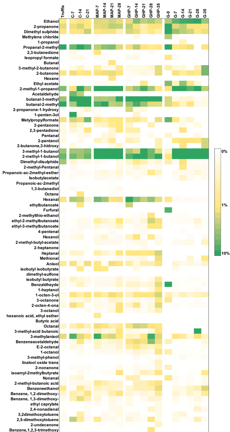
Fig. 4. Heatmap of the volatile profile of truffle and gelatine samples according to the relative percentage of area values detected using SPME-GC-MS. Samples were fresh truffle (truffle), truffles with control packaging (C), truffles packaged in modified atmosphere (MAP), truffles in gelatine hydrogel-based package (GHP), and gelatine from GHP samples (G). The numbers (7, 14, 21, 28 and 35) correspond to the different storage days of the experiment.
