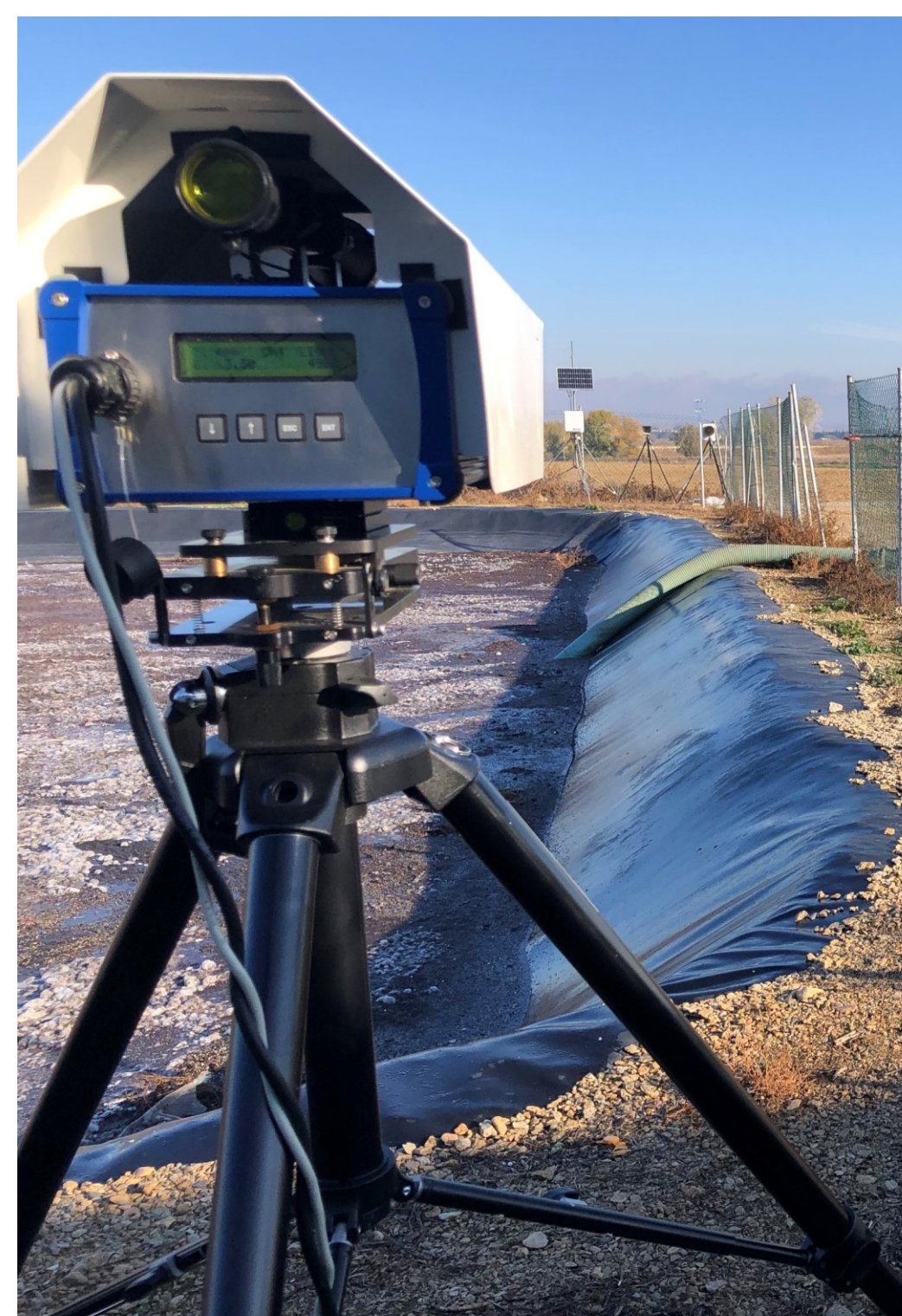
Fig.1. Gas analyser measuring air CH 4 concentration over the lagoon.
