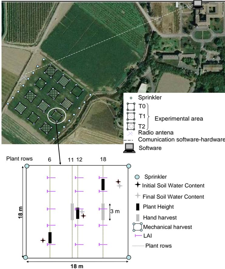
**Figure 1.** Aerial photograph of the field experiment, detailing the location the software application, the hardware and the radio antenna. The experimental design (three treatments, four replicates) is presented. The location of the measurement points within an experimental plot is also presented
